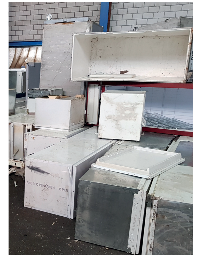
Photo 2: Refrigerators prior to being processed at stage 2 (shredding with recovery of propellants).
