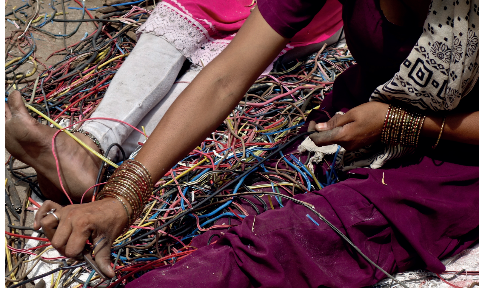
Photo 1: Skinning of cables and colour-sorting of fractions in the informal sector in Delhi, India.
